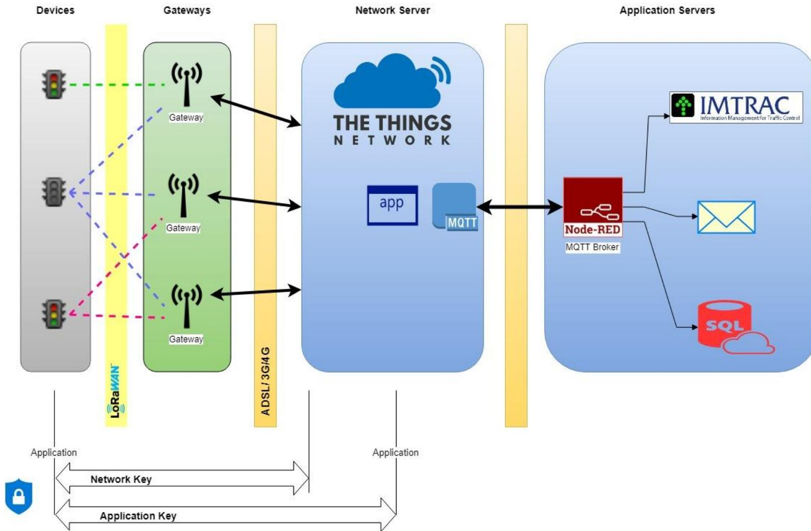
Figure 1 LoRaWAN network architecture and security
